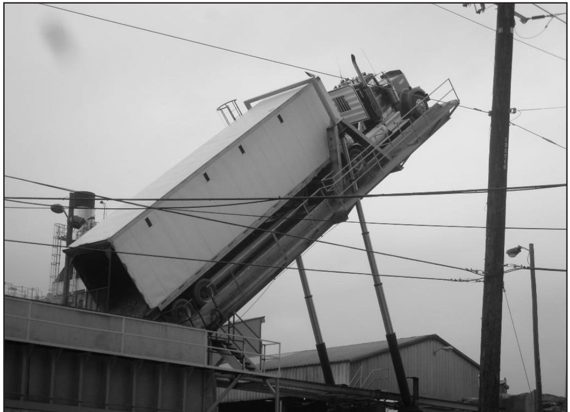
An 18-wheeler is lifted by a huge hydraulic platform to dump its contents of wood chips at the Multitrade biomass plant in Rabun Gap, GA. At full capacity, the plant will burn up to 50 tractor trailer loads of wood chips per day.
