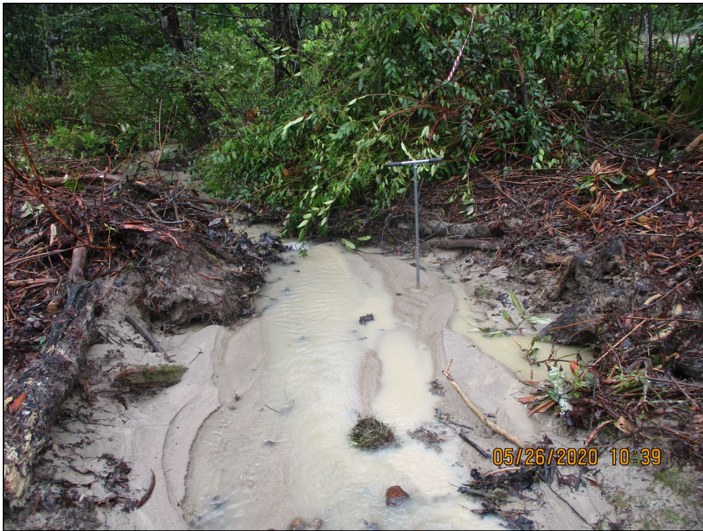
Photo 3: Flag S4, 6-12 inches of sediment accumulated in stream bed. View downstream.
