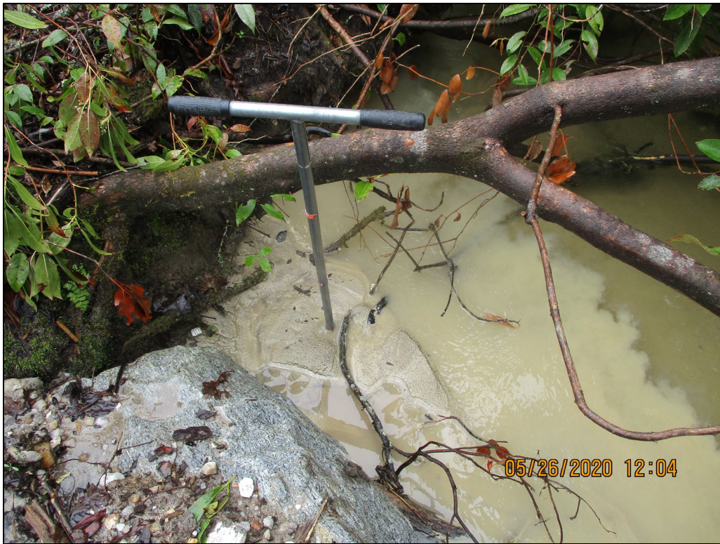
Photo 5: Flag S9, 12 inches of sediment accumulated in stream bed. View downstream.
