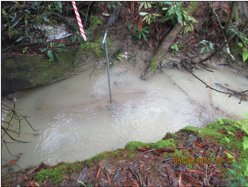
Photo 1: Flag S1, 6 inches of sediment accumulated in stream bed. View toward left bank.
