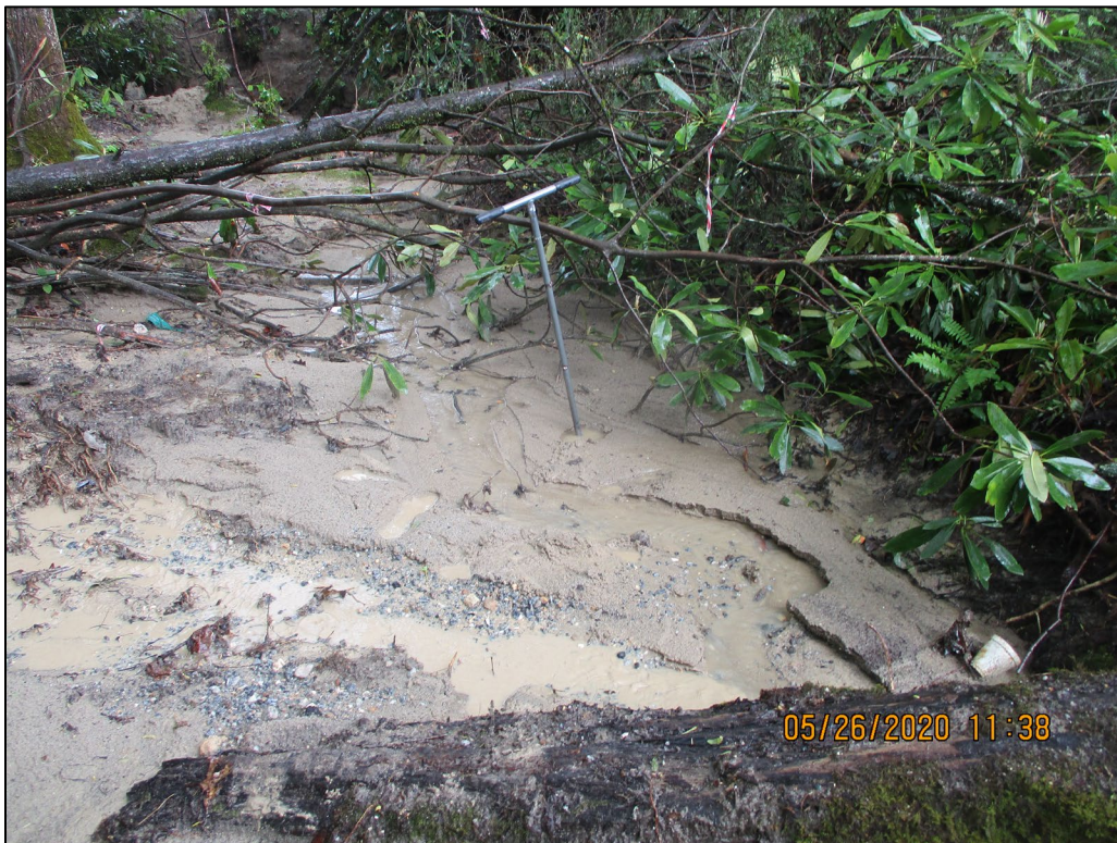
Photo 4: Flag S7, 12 inches of sediment accumulated in stream bed. View upstream.
