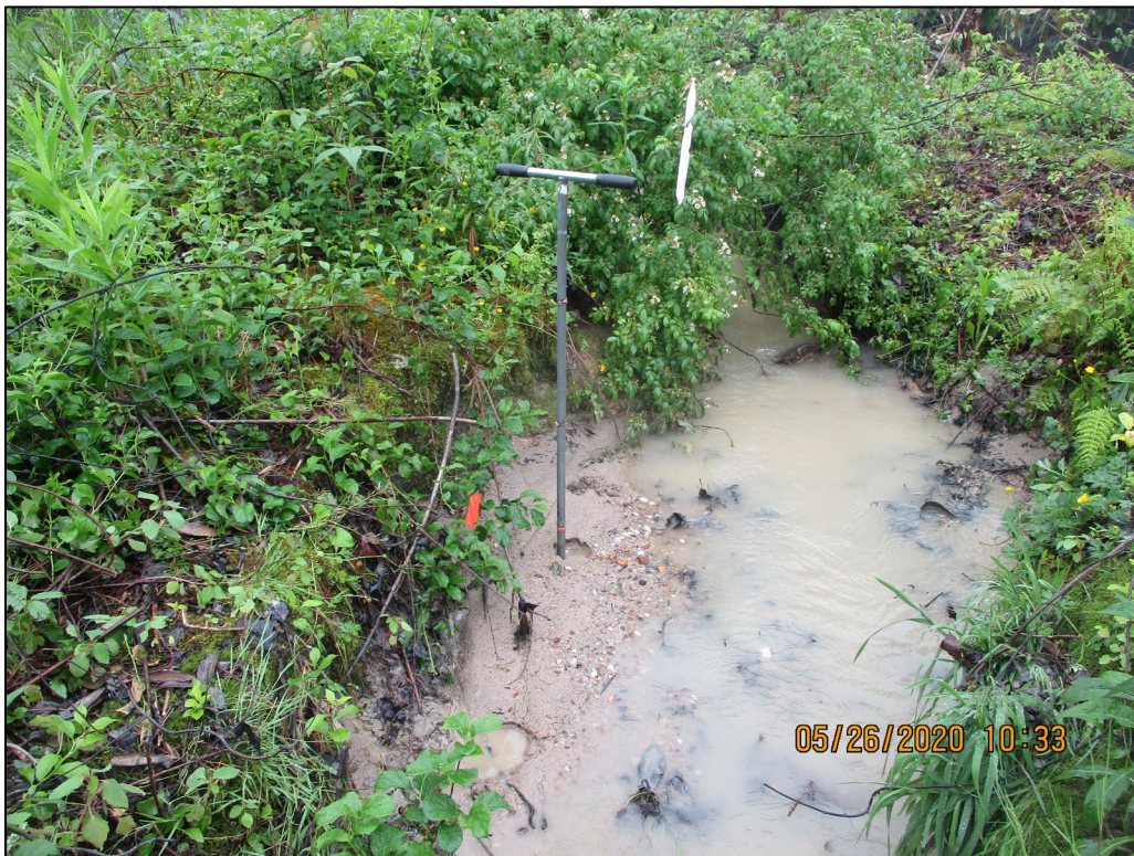
Photo 2: Flag S3, 8 inches of sediment accumulated in stream bed. View downstream.
