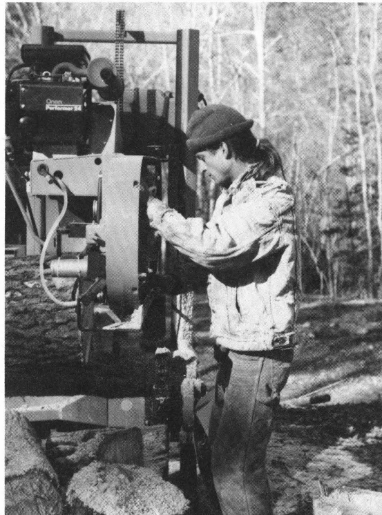
Portable band mill - no haul cost and little waste.
