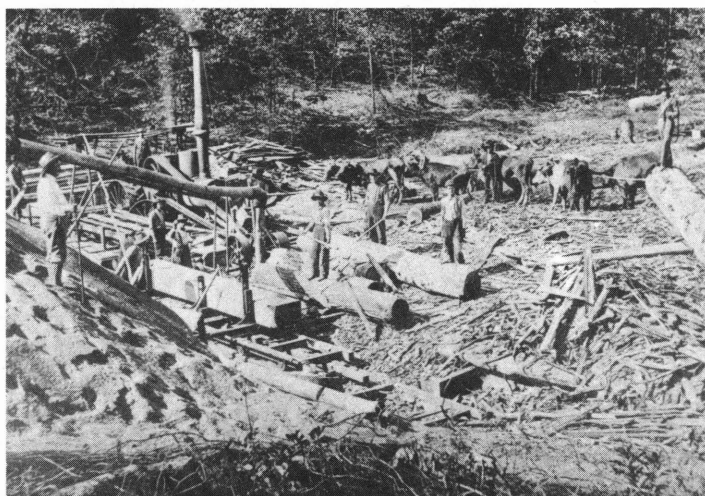
Steam powered sawmill on the Chattooga.
