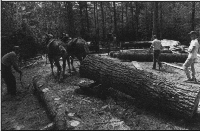
Mike and his team of Belgian draft horses drag a large white pine to the portable bandsaw on the log deck.
